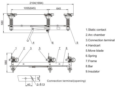
Drawing 1 12kV Switch structure (closing)
