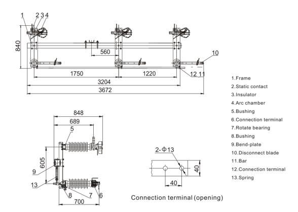
Drawing 3 40.5kV Switch structure (closing)
