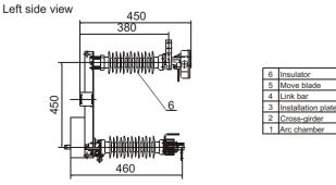
Drawing 2 24kV Switch structure
